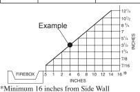
Figure 8 - Minimum Clearance for Combustible to Wall
